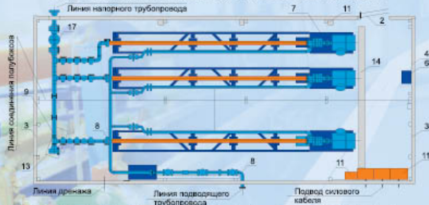
Station's overall view: 1 – mobile container, 2 – entrance door, 3 – service entrance, 4 – gates, 5 – electric heater, 6 – service table, 7 – pump unit УЦ 250-1600, 8 – feed pipeline, 9 – pressure pipeline, motor switchboard, 11 – controller, 12 – overhead crane, 13 – discharge tray, 14 – cable duct, 15 – electrically-driven valve gate, 16 – return valve, 17 – electrically-driven control valve gate
