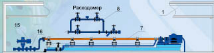
Station's overall view: 1 – mobile container, 2 – entrance door, 3 – service entrance, 4 – gates, 5 – electric heater, 6 – service table, 7 – pump unit УЦ 250-1600, 8 – feed pipeline, 9 – pressure pipeline, motor switchboard, 11 – controller, 12 – overhead crane, 13 – discharge tray, 14 – cable duct, 15 – electrically-driven valve gate, 16 – return valve, 17 – electrically-driven control valve gate
